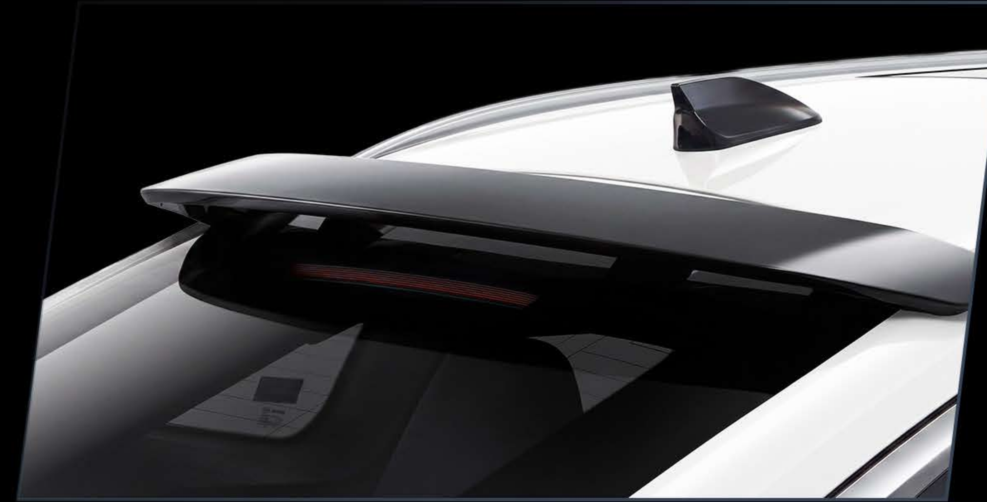
➤ Roof spoiler trim to optimize airflow and increase downforce
